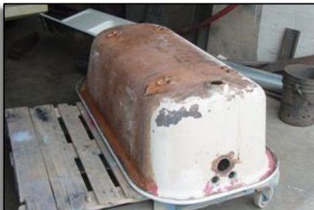
Rusted clawfoot tub will need sandblasting before refinishing. These have often been painted many times and probably have lead paint from the early 1900's
